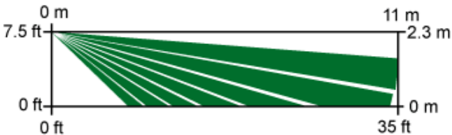
Side View Standard Broad Coverage 11 m x 11 m Walking speed range is 0.2 m/s to 3.0 m/s
